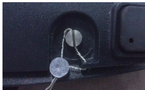
Locked with Wire Seal
